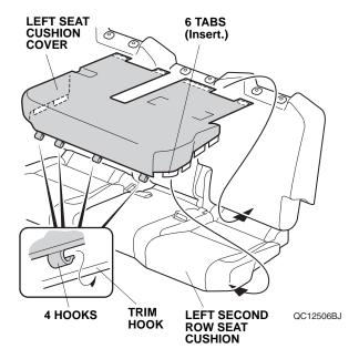
Set the left seat cushion cover under the seat belt buckle as shown. Insert the left seat cushion cover between the left second row seat-back and left second row seat cushion, and secure the fasteners to the left second row seat cushion.
