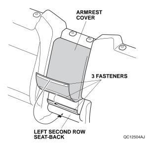
Secure the fastener to the bottom of the left second row seat-back.
