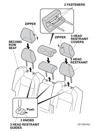
2. Fit three head restraint covers over the head restraint, and secure the fasteners and the zippers on the head restraint covers as shown.
