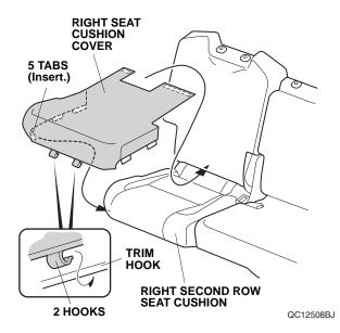
Insert the right seat cushion cover between the right second row seat-back and right second row seat cushion, and secure the fasteners to the right second row seat cushion.
